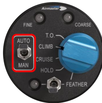
Figure 2. Control Mode Selector (AC200 feathering controller shown).
