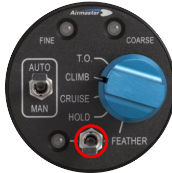
Figure 4. Engage Switch (AC200 feathering controller shown).
